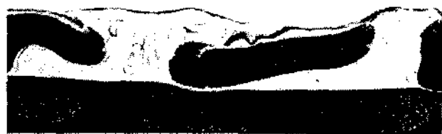
Figure 20. Cross section of silicone domes with strongly folded sheets of modelling clay.
